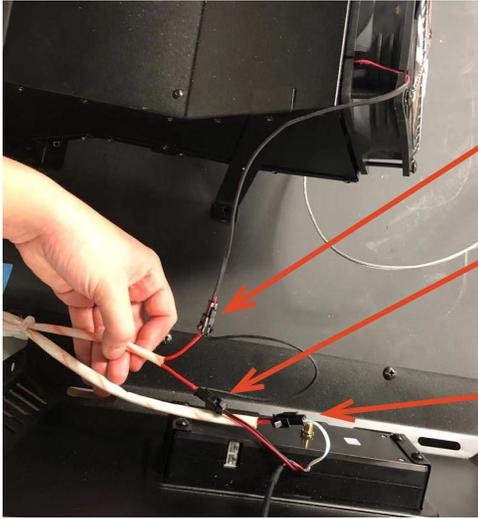
The “black only” wire coming from the fan is connected to one of the “red only” wires coming from the body of the smoker.
