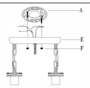
5. Carefully pass wires through the mounting plate assembly (A) Secure the mounting plate assembly (A) to outlet box with the mounting screws (D).
