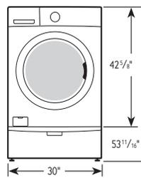
Required Dimensions for Installation with Stacking Kit
