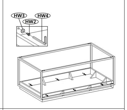
Step 1: Put the Flat washer(HW3) on the Hex bolt(HW1), insert the Crossbeam(B and C) into Leg frame(D) in order. Insert the Hex bolts into the mounting position and tighten them by using Allen key(HW4).
