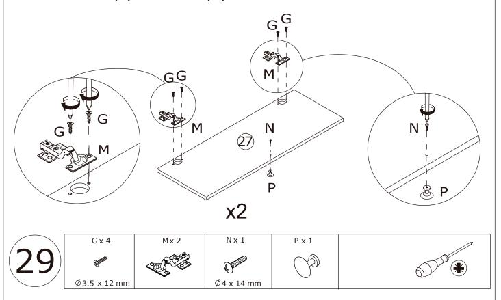
Fix hinge(M) to plate 26 with screw(G), fix knob(P) with screw(N) as shown.
