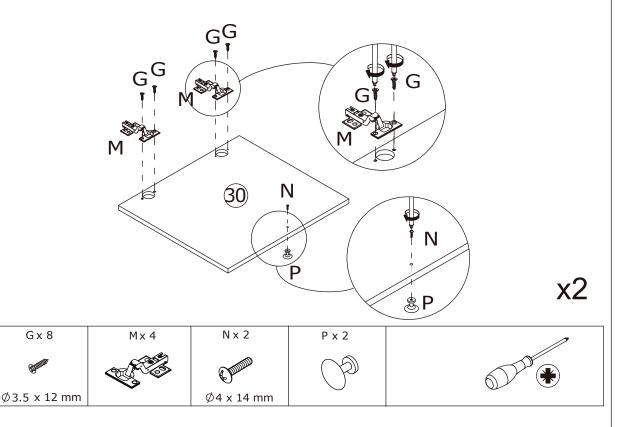
Fix hinge(M) to plate 28 and 29 with screw(G), fix knob(P) with screw(N) as shown.
