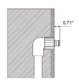
14. Place the trim plate onto the hand shower armand secure the hand shower arm to the connector.
