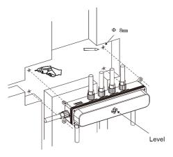
2. Wrap telon tape around the threads of the male adapters and connect the hot, cold, shower head, hand shower and back spray head water lines to the valve body.
