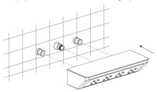
23. Tighten the two M5 screws to secure the back spray head.
