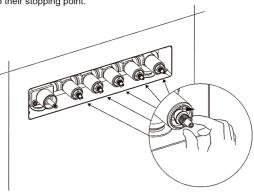
5. On the back side of the valve trim panel, run a bead of silicone around the edge and placeit onto the valve body securing it to the finish wall.
