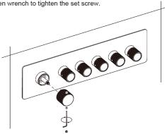
7. Insert the push button connectors into the knobs and secure.
