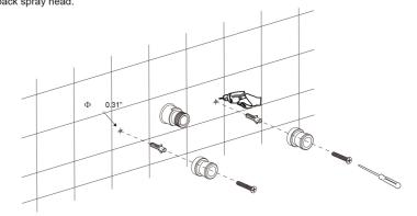
22. Install the back spray head onto the outlet connector and mounting adapters.
