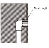
19. After verifying the center of the water outlet and distance needed for the mounting adapters mark the locations ensuring that both marks are level.
