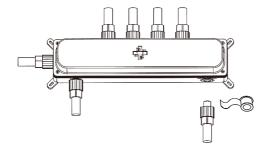
3. After the wall is finished, remove the plastergaurd from the valve body and cut the valve body casing flush with the wall if necessary. Discard the platergaurd.
