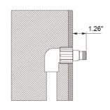
21. Drill out the two marks and secure the mounting adapters to the finish wall.
