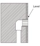
13. Wrap the threads of the hand shower arm connector and screw it into the wall connection, as shown in the images.
