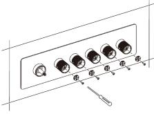
8. Insert the push buttons caps onto the diverter knob connectors making sure that they are even with the end of the knobs.
