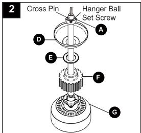
3. Hanging the fan motor assembly to the mounting bracket.
