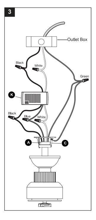
After connecting the wires, spread them apart so that the green and white wires are on one side of the outlet box and the black and blue wires are on the other side. Carefully tuck the wire connections up into the outlet box.
