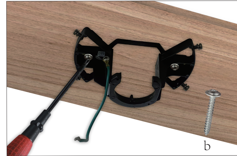
Step 1 For wooden ceiling, install the hanging bracket to wooden ceiling with two wood screws.
