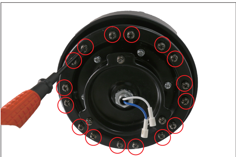
Step 13 Remove the screws which are used to install Blades.
