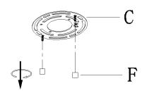
6. Attach the mounting plate (C) to outlet box with the mounting screws (B).
