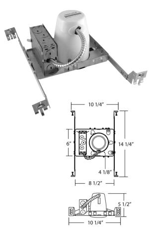
Suitable for new construction in residential and commercial applications. NON-IC. Insulation must be kept a minimum of 3" from housing.
