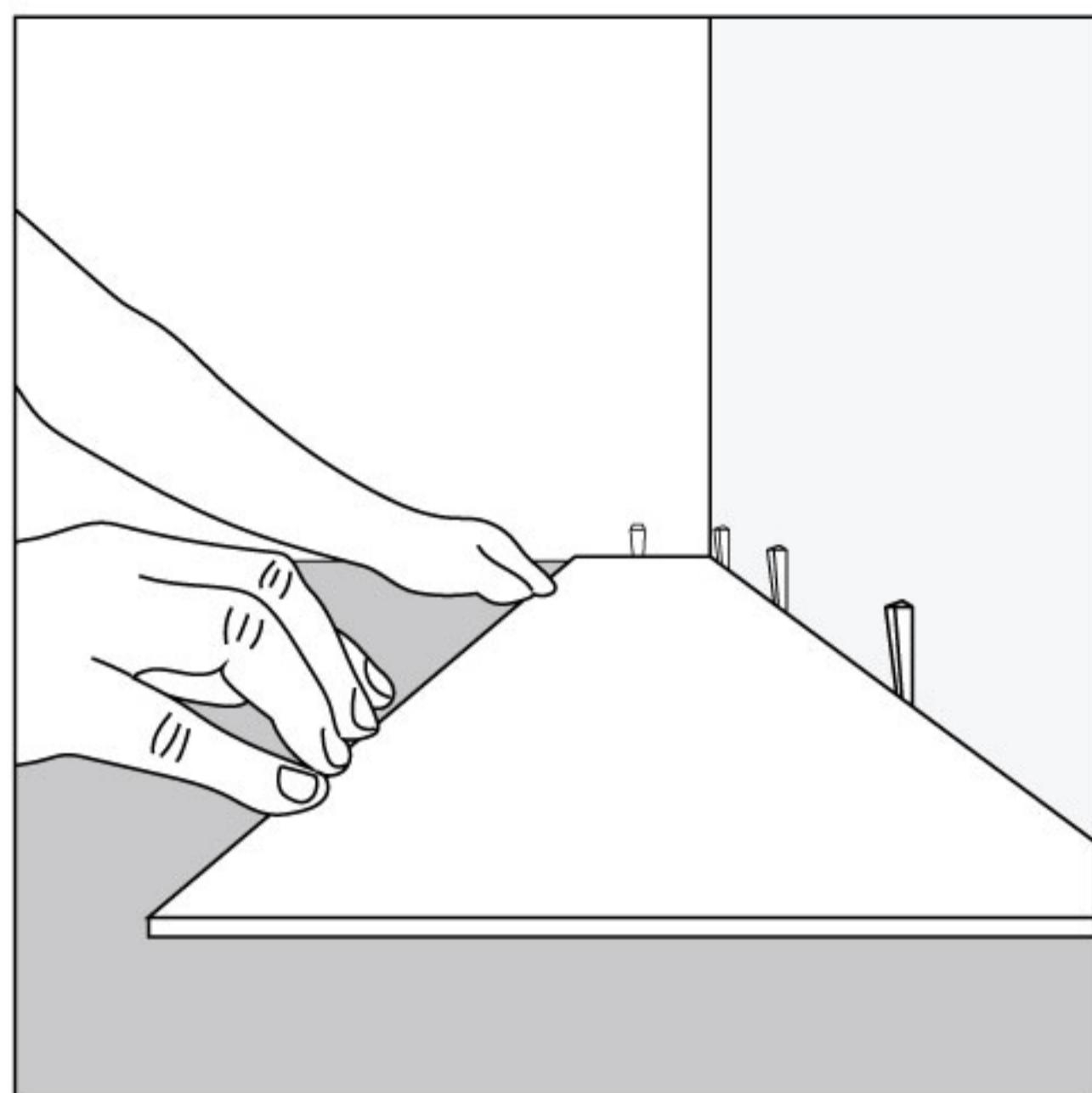
After thoroughly cleaning the subfloor, install the 6-mil poly underlayment. Then you should begin laying in the left-hand corner. Place the floorboard 1/4" from the left wall. Use spacers between the wall and the floorboard.
