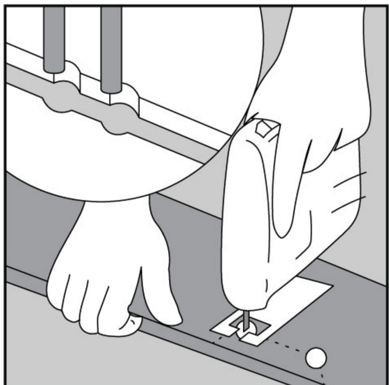
Holes for pipes: measure the diameter of the pipe and drill a hole that is 7/8" larger. Saw off a piece as shown in the figure and lay the board in place on the floor. Then lay the sawed-off piece in place.
