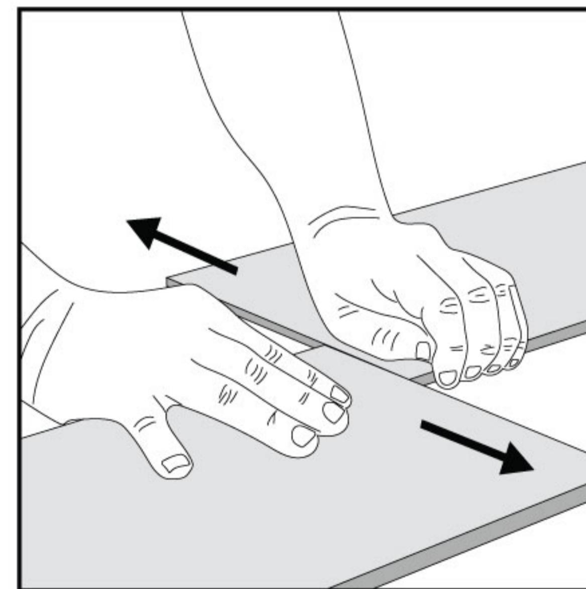
Separate the whole row by lifting it up delicately at an angle. To separate the planks, leave them flat on the ground and slide them apart. If planks do not separate easily, you can slightly lift up the planks ( $5^\circ$ ) when sliding them apart.
