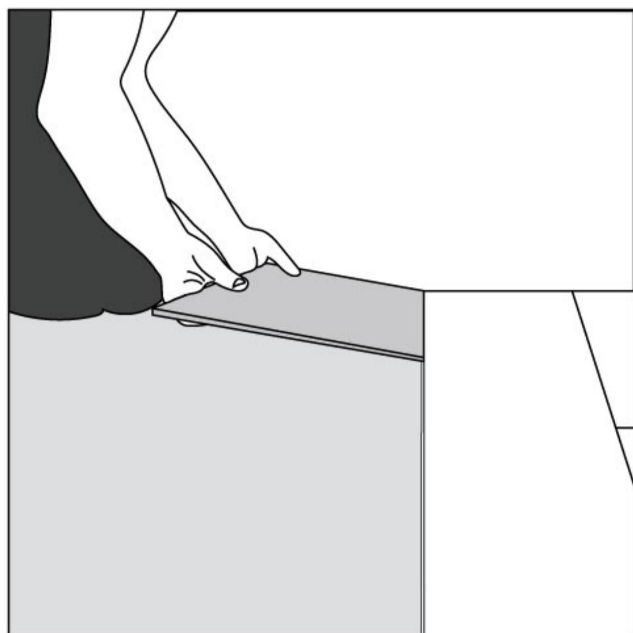
Second Plank, first row. Drop the plank and gently press down the end with a rubber mallet so it firmly locks into the previous plank until both are at the same height. Make sure both planks are perfectly aligned. NOTE: If you notice both planks aren't at the same height or are not well locked together, please follow the disassembling instructions at the bottom of the page, disassemble and check if any debris stuck inside the lock is obstructing.
