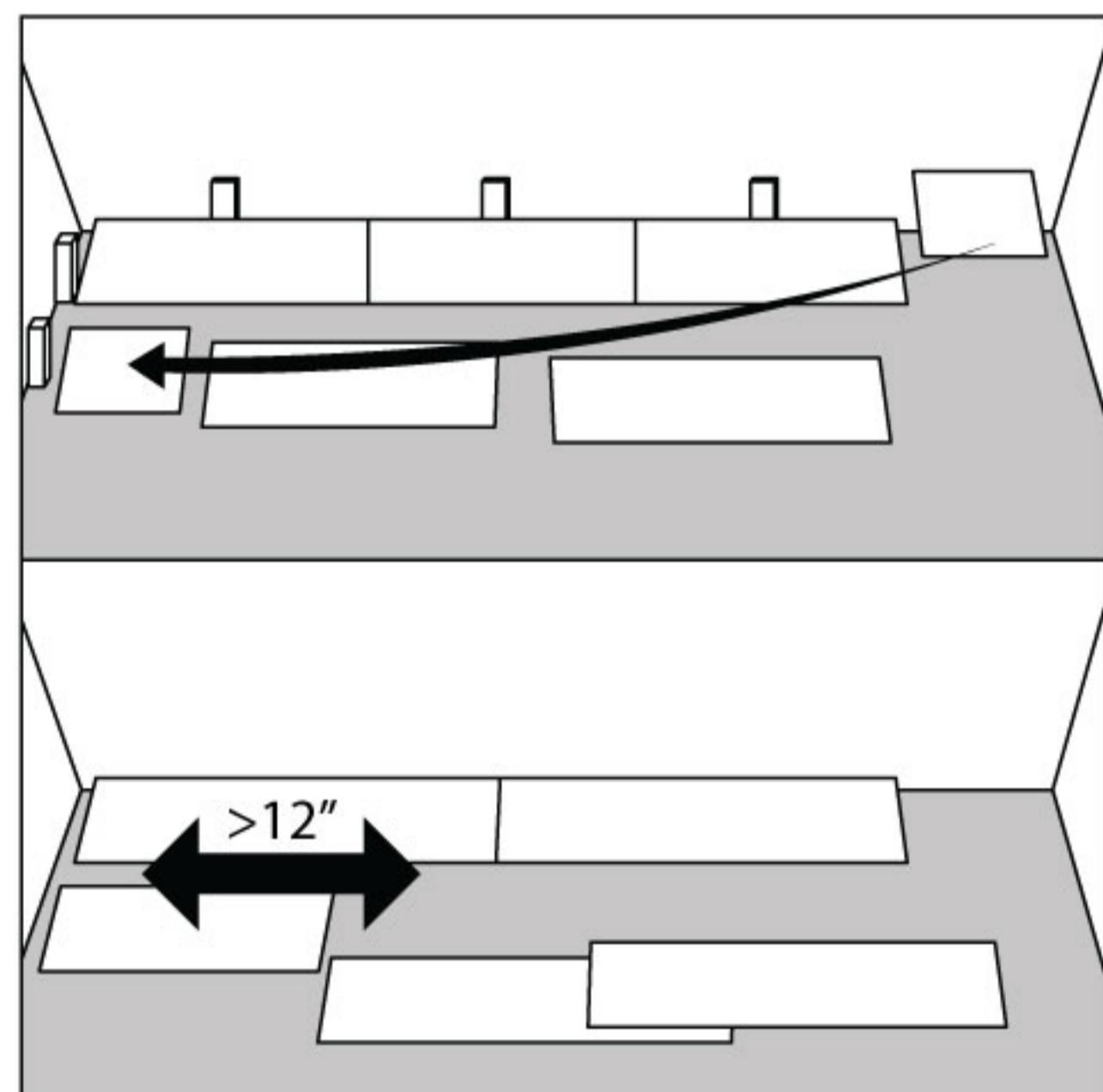
Start the second row with the leftover cut part of the last plank of the previous row. This small plank should measure at least 12". Otherwise, use another plank that should be cut in two. The end joints of each adjoining row should not be closer than 8" to each other.
