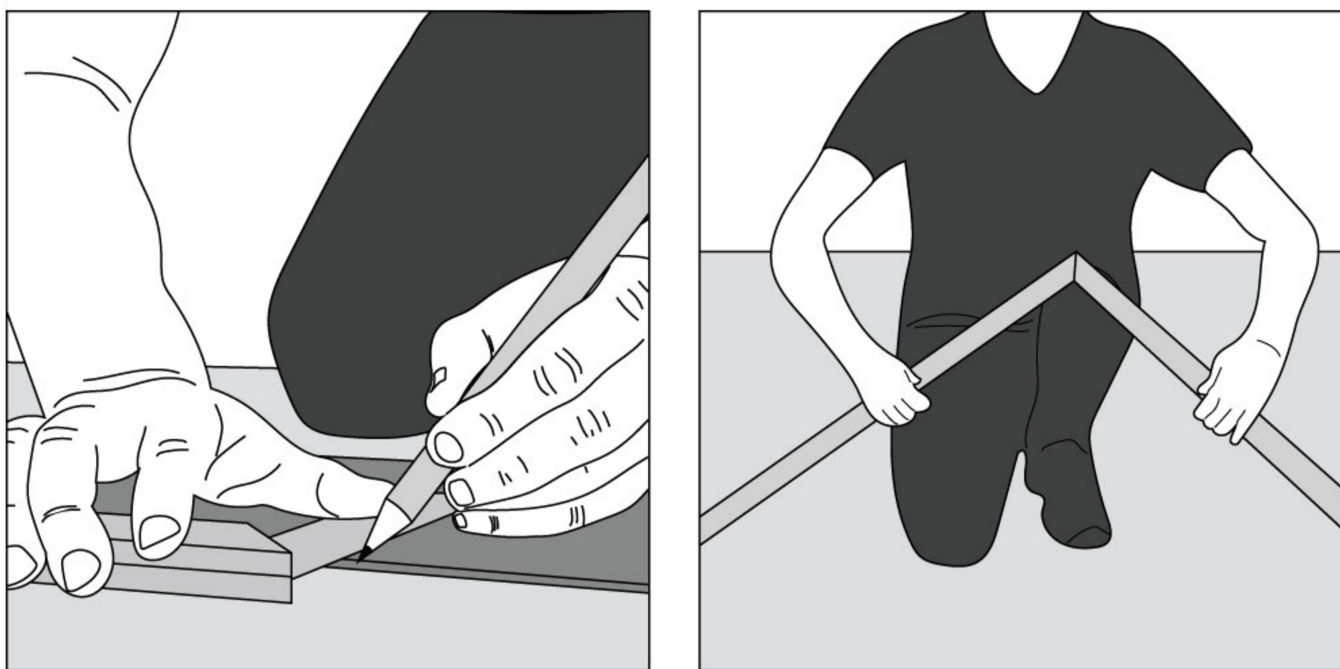
To cut the plank, use a simple utility knife and ruler, and with the top side facing up, cut heavily and several times on the same axis. The knife will not go through the surface but make a deep cut. You can then lift one half of the plank using your other hand to hold down the second placing it very close to the cut. The plank will split naturally.
