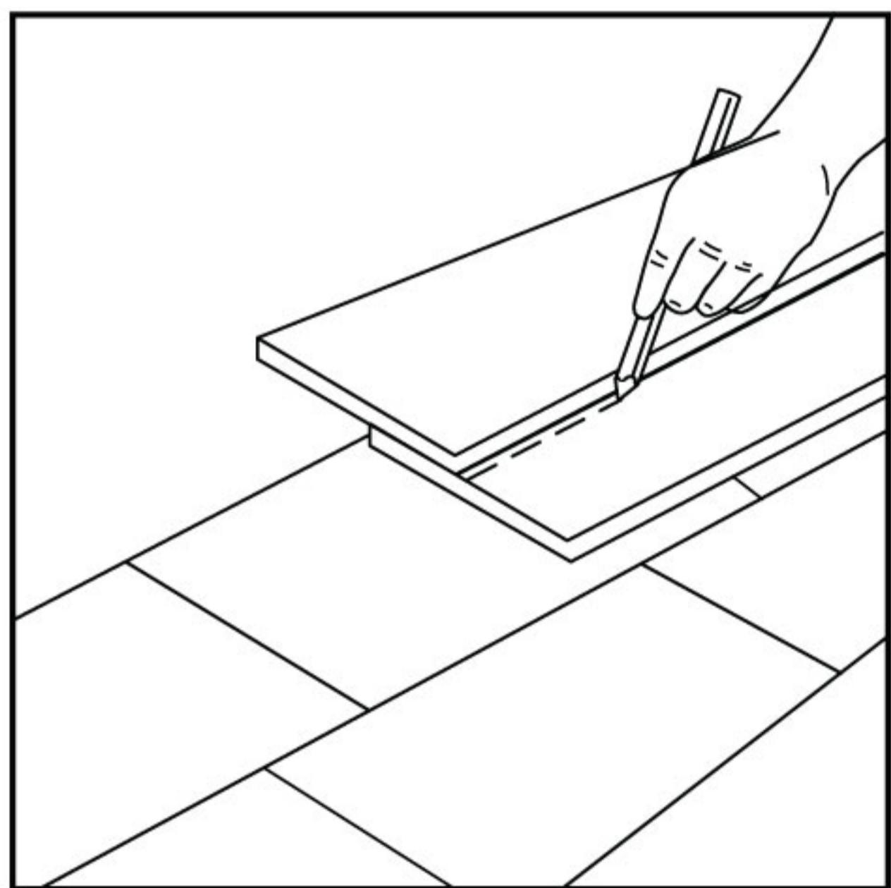
To lay the last row: position a loose board exactly on top of the last row laid. Place another board on top, with the tongue side touching the wall. Draw a line along the edge of this boards, to mark the first board. Cut along this line to obtain of the required width. Insert this cut board against the wall. The last row should be at least 2" wide. The spacers can then be removed.
