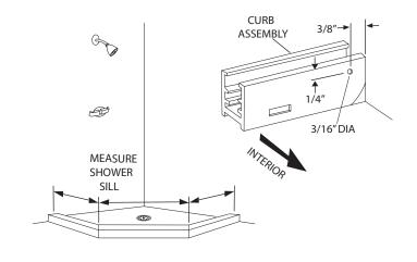
Place the two wall jambs [E] into the ends of the curb assembly [A]. Plumb the jambs and mark the hole locations on the wall. Masking tape may be used to hold the curb in place during this operation. Remove all parts and drill the walls for mounting hardware.
