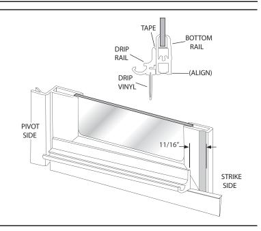
Adjust the drip vinyl [T] by sliding it left or right until it almost touches the curb. Trim the vinyl (flush with the pivot end and notch 1/4" longer than the drip rail as shown on the strike end).
