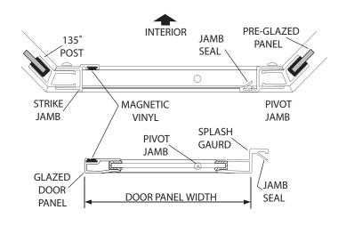
Snap the fillers [P] into the curb assembly [A] and header assembly [D] between the door jambs with the RAISED LIP TO THE EXTERIOR and the pivot holes toward the pivot jamb [M]. Center the curb filler in the curb between the pivot and strike jamb [N] (use masking tape to hold in position).
