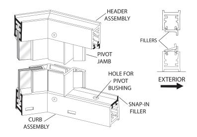
Pull the bottom end of the pivot jamb [M] tight to the curb filler [P] and plumb the jamb. Drill two 1/8" holes thru the pivot jamb and into the 135° post [J] in line with the screws in the head and curb and approximately 1/4" vertically from the ends of the jamb. Drill a third hole centered between the first two. Attach the pivot jamb permanently with three #8 x 1/4" truss head screws [C].
