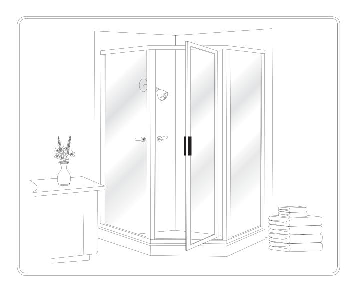
**MAINTENANCE:** Two primary materials are used to manufacture your new Basco enclosure: tempered glass and anodized aluminum. To assure a long lasting finish on the enclosure, wipe it down with a towel after each use. Never use a scouring agent to clean the aluminum.
