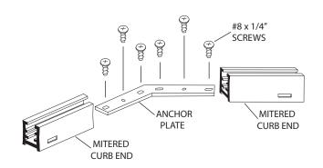
The curb should sit near the centerline of the sill. If required, use a file to round the lower ends of the curb assembly to fit the shower sill properly.
