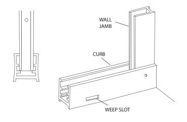
Wipe the shower walls and sill, curb assembly [A] and wall jambs [E] with a clean, dry cloth to remove any dust or debris. Apply a 1/4" bead of caulk along the inside of both of the pencil lines marked in Step #3. Carefully replace the curb assembly in the exact position marked. Caulk the inside of the curb ends where they meet the wall. Caulk around the anchor plates [B], screws [C], and the insides of the mitered joints.
