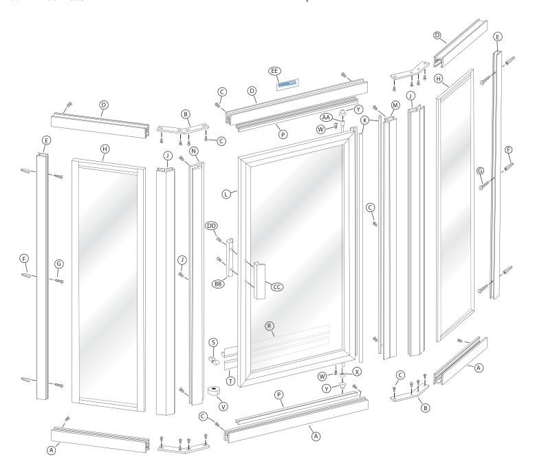
The BASCO 160 Quick-N-Stall Shower Enclosure is completely reversible and may be installed pivot-left or pivot-right. For maximum waterproofing, the pivot jamb should be opposite the shower head. Using the diagram, determine the correct position for the door in your particular Quick-N-Stall installation. This instruction sheet depicts a pivot-right installation.
