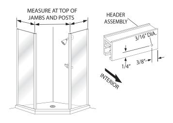
Press the header assembly [D] over the wall jambs [E], the 135° posts [J] and the pre-glazed panels. Check the posts for plumb. Adjust as required by varying the overlap of the header over the wall jambs. You may need to trim the ends of the header where it meets the wall. The minimum horizontal dimension for the door opening is the door panel width (see the graphic in Step #9) plus 1/2", maximum is the door panel width plus 1 3/4".
