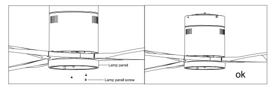
Unscrew a set screw. Attach the LED pan up to the bottom of the fan by inserting the other two set screw heads into key hole slots, rotate it to place, then secure the previous set screw by aligning screw hole and the hole at the bottom of the fan, tighten the rest two set screw to secure LED pan.
