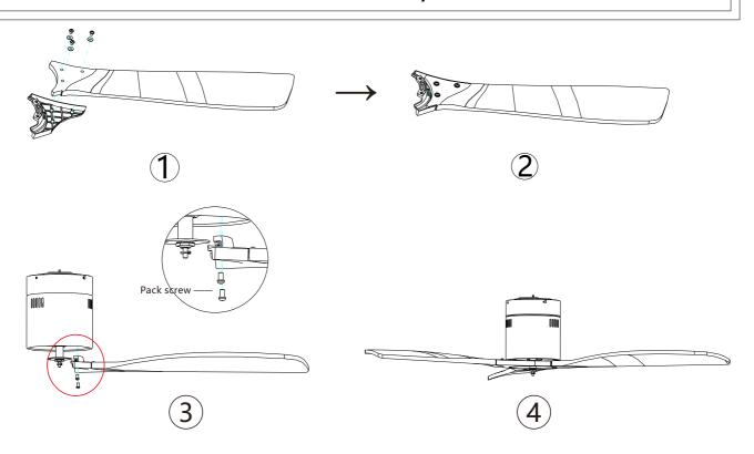
Align the blade holes with the motor screw holes, tighten the screw and secure all blades.
