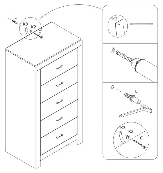
Install anti-tipping device as shown.
