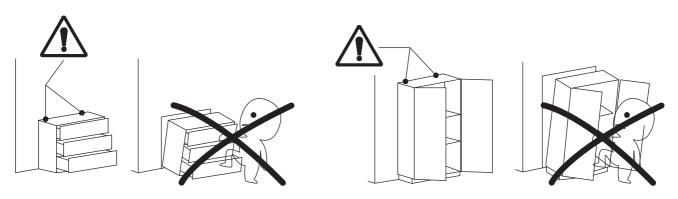
Once assembled lift furniture into place, do not drag. Use a drill to create a small hole lining up with the top of the safety strap (K3). Fasten to wall using wall anchor (L), washer (K2), wall screw(C). Ensure the unit is balaced and steady before use. You're done, enjoy
