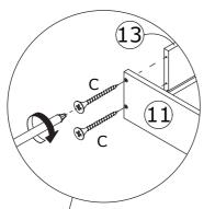
Fix board 11, 15 and 12 to board 13 with screw(C) as shown. Insert back board 14 along grooves as shown.
