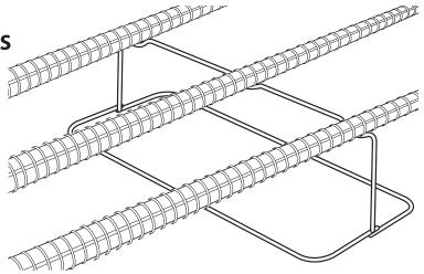
3 Secure rebar in place with tie wire
