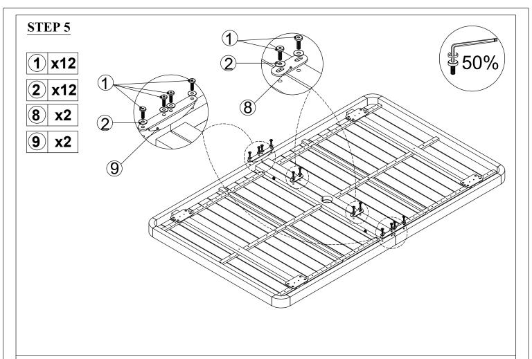
Connect the part from step 4,with Midle Connector (8), Side Connector (9), Tighten Bolt (1) & Flat Washer (2) with Allen Wrench (10).
