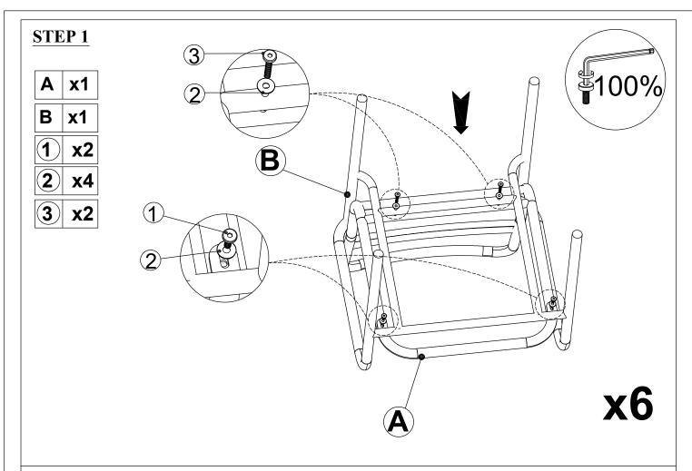
Connect Seat Chair (B) & Back Chair (A), Tighten Bolt (1), (3) & Flat Washer (2) with Allen Wrench (10).
