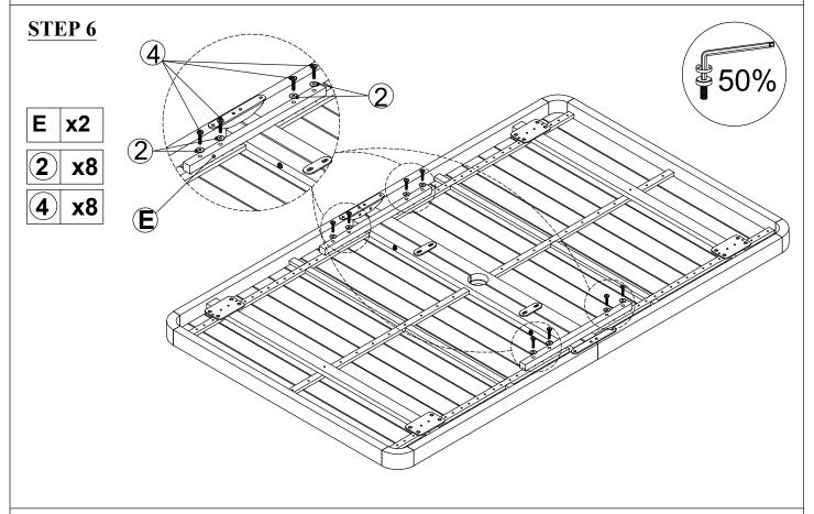
Connect the part from step 5,with Connector (E),Tighten Bolt (4) & Flat Washer (2) with Allen Wrench (10).
