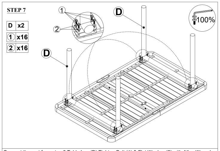
Connect the part from step 6,Table Leg (D),Tighten Bolt (1) & Flat Washer (2) with Allen Wrench (10).
