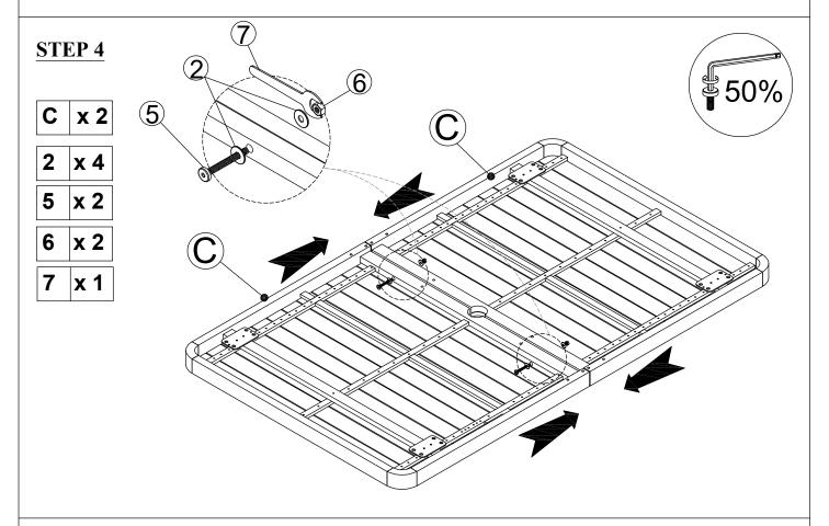
Connect Top Table (C) Tighten Bolt (5) & Flat Washer (2) & Nut (6), Key (7) & with Allen Wrench (10).
