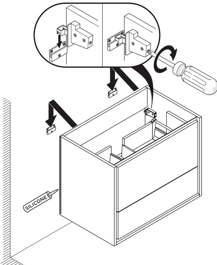
**4** Apply a bead of silicone on the top of the cabinet and place sink on the cabinet
