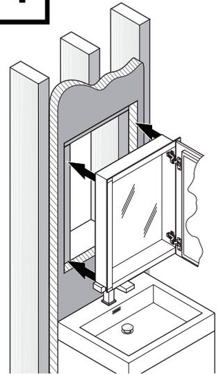
Cut the marked perimeter with appropriate tool.
