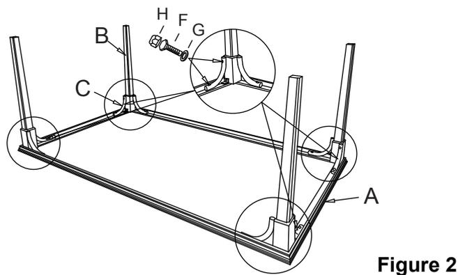
Step 4. Check the alignment and adjust if necessary. Once the alignment is correct, tighten all bolts with open wrench ( I ). Cover all bolts with bolt caps(H).
