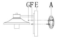
2) Uncrew the ball knobs (G)from the top of frame(I). Then align the holes in lid with nipples on the top of frame(I), secure with gasket (F) and ball knobs(G)
