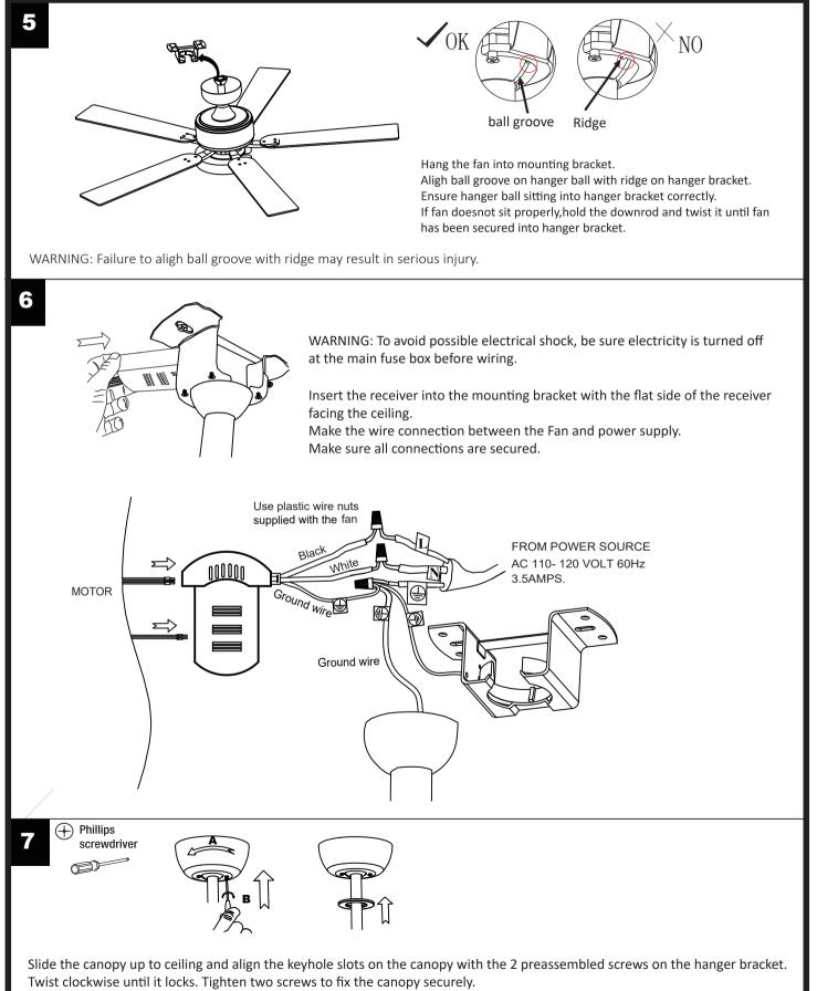
Clip the canopy cover in to secure it onto the canopy.
