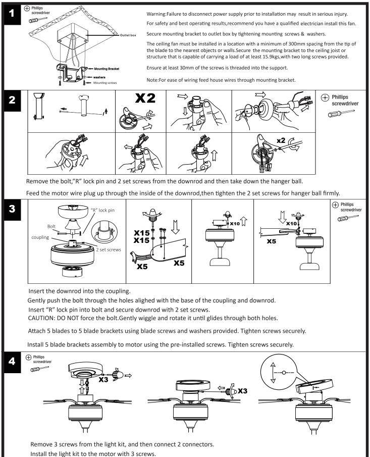
The light kit can be adjusted the direction.
