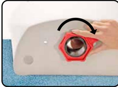
**B:** Apply red tank-to-bowl gasket to bottom of flush valve locknut, fully covering locknut.
