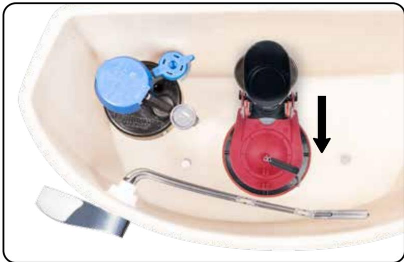
**NOTE: Do not** cover tank bolt holes with flush valve. If flush valve covers a bolt hole, turn flush valve slightly to the right (overflow tube to the right) to clear the bolt hole. In some cases, placing bolts in the holes first may be necessary.
