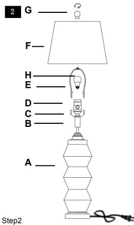
Insert the Harp (E) into the Saddle (C). Put the shade(F) on the Harp(E),then tighten the Finial (G)into the Harp (E) Insert the bulb(H) into the socket(D).
