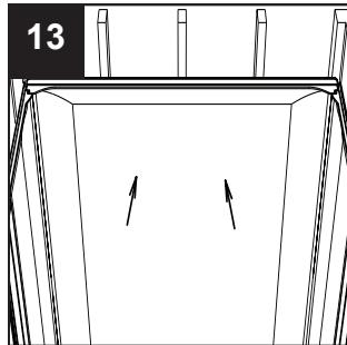
14. Install and caulk (not included) around all holes for faucet, diverter valve and showerhead (not included).
