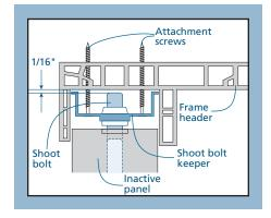
end of the shoot bolt and the frame header. If necessary, perform shoot bolt height adjustment.
