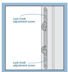
latch and two adjustment screws.
