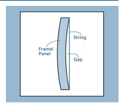
3. Look for gap between string and frame or panel. If gap measures more than 1/16" at any point, the panel is bowed.
