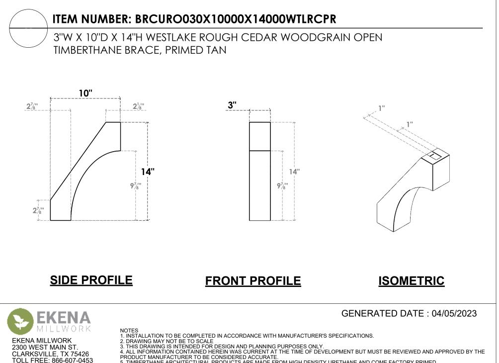
5. TIMBERTHANE ARCHITECTURAL PRODUCTS ARE MADE FROM HIGH DENSITY URETHANE AND COME FACTORY PRIMED
