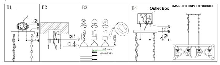
STEP B1: Unscrew the ball knobs (H) from canopy (E) then gently remove the mounting plate assembly (B) STEP B2:Carefully pass the outlet box wires through the mounting plate(B), then secure the mounting plate assembly (B) to outlet box with the mounting screws(C).
