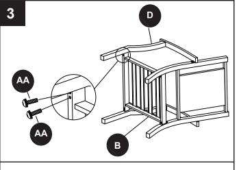
Hand tighten AA. Do not tighten with wrench BB, until all bolts have been installed.
