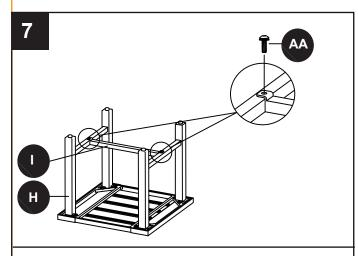
Once all bolts have been installed and hand tighteded, go back and tighten firmly.
