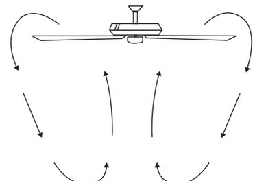
**NOTE:** To operate the reverse function on this fan, press the reverse button while the fan is running at any speed.
