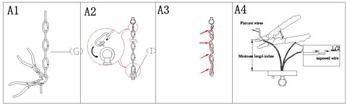
Step A1: By measuring, determine the correct length of wires needed. Use the wire pliers, cut and discard the remaining wires.
