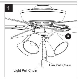
2. Using a ceiling fan will allow you to raise your thermostat setting in summer and lower your thermostat setting in winter without feeling a difference in your comfort. **Note:** Wait for the fan to stop before moving the reverse switch located on the light kit (G).
