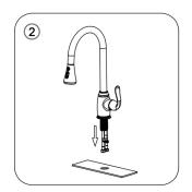
2. For single hole installation insert the hot and cold supply lines and shank through the hole in the countertop.
