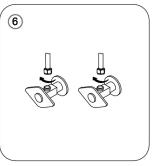
6. Connect the open ends of the hot and cold supply lines to the shut off vales. Ensure the faucet is in the off position and turn on shut off valves. Check for leaks.
