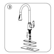
3. For a 3-hole installation insert the base plate panel into the base plate and slide it onto the faucet shank. Insert the hot and cold supply lines, spray hose and shank through the hole in the countertop.
