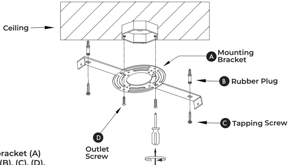
Secure mounting bracket (A) with outlet screws (B), (C), (D).
