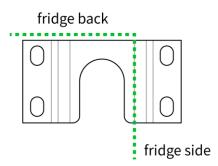
4. While the brackets are in position on the floor, mark the position of all 4 holes on each bracket. Before drilling any holes, double check all measurements and place the fridge near the brackets to check your accuracy. Bracket openings should line up with the adjustable feet on the back of the unit. Use a 5/16 drill bit to make holes for the plastic anchors. Insert the plastic anchors.
