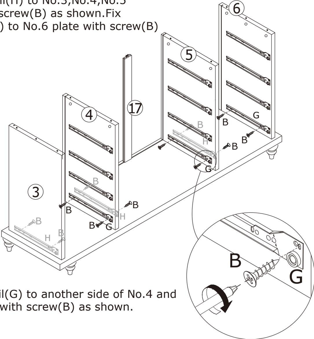
Fix slide rail(G) to another side of No.4 and No.5 plate with screw(B) as shown.
