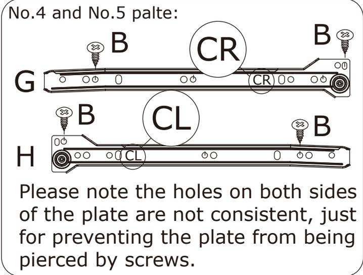
Fix slide rail(H) to No.3, No.4, No.5 plate with screw(B) as shown. Fix slide rail(G) to No.6 plate with screw(B) as shown.
