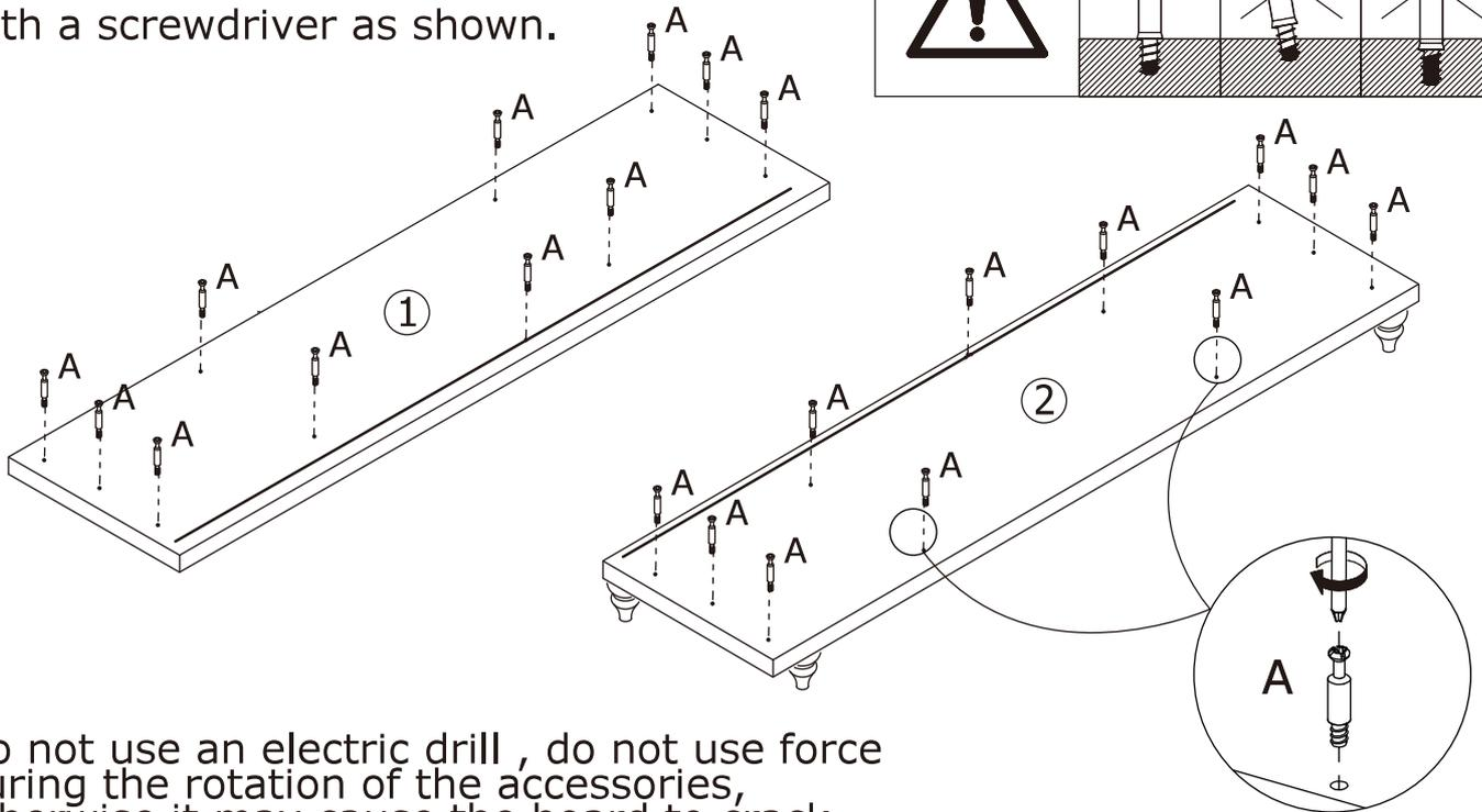
Do not use an electric drill , do not use force during the rotation of the accessories, otherwise it may cause the board to crack.
