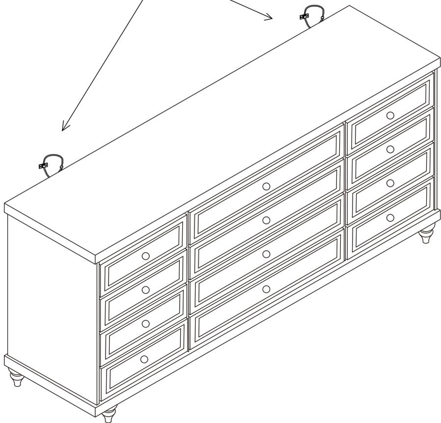
Fix part(Q) to No.1 plate with screw(T) at first.
