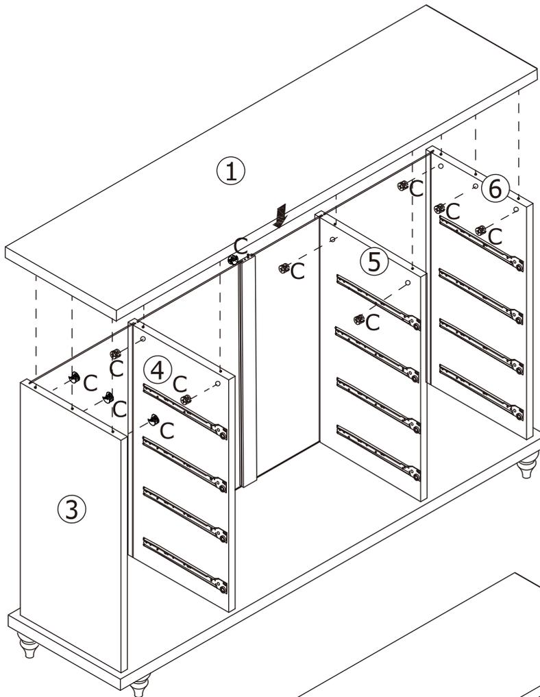
Cover No.1 plate to the top the unit, then turn cam lock(C) in No.3,4,5, 6 plates clockwise to tighten as shown.
