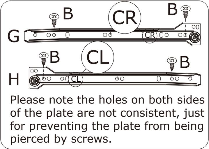
Please note the holes on both sides of the plate are not consistent, just for preventing the plate from being pierced by screws.
