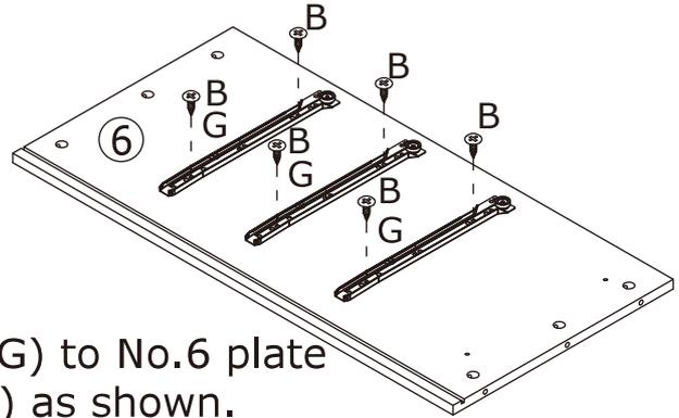
Fix slide rail(G) to No.6 plate with screw(B) as shown.
