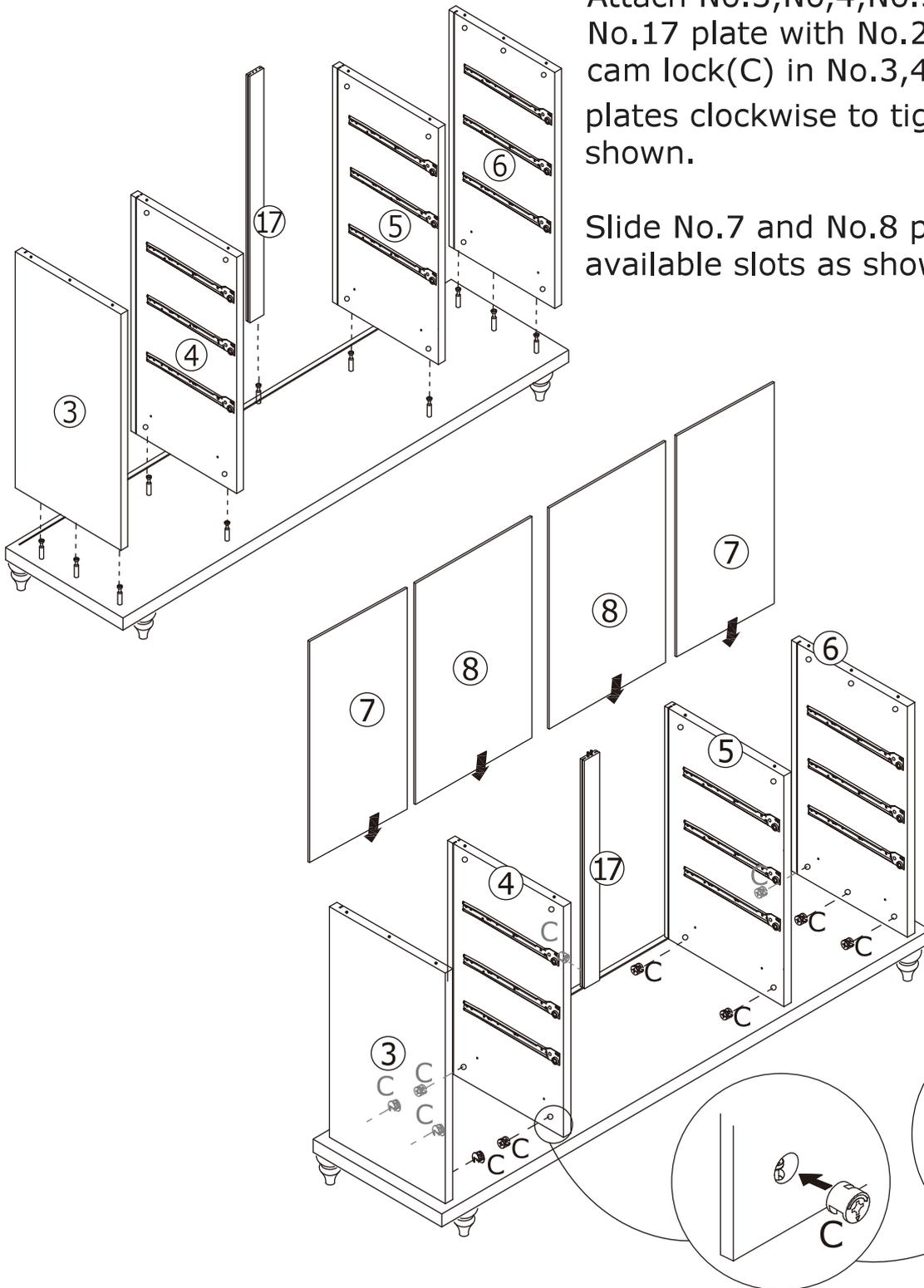
Attach No.3, No.4, No.5, No.6 and No.17 plate with No.2, then turn cam lock(C) in No.3,4,5,6,17 plates clockwise to tighten as shown.
