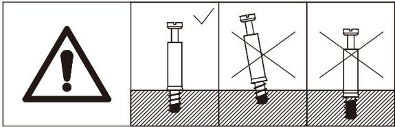
Insert quickfit screw(A) into No.10 plate and No.20 plate with a screwdriver as shown.
