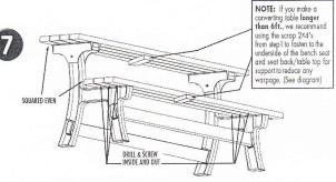
To make the seat, position the first of the remaining three 2x4's at the front edge of the Bench Ends, and squared with the table top. Fasten underneath through the screw slots, inside and out, with 12 of the screws provided. Position and fasten the last (2) 2×4's, squared and spaced about 1/4" apart.
