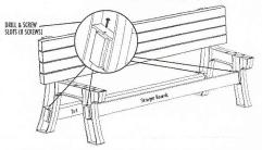
Align the ends of the stringer boards **flush to the end of the holes** in the legs of the Bench Ends. Drill pilot holes into 2x4's at **all** of the screw slots, inside and outside, of both legs and fasten with 8 of the screws provided.
