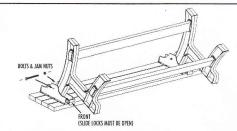
Make sure the Slide Locks are in the open position and the front (open slide
