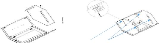
The two optional hanging bars are included. These are to be installed at the top and bottom of the inside of the cabinet prior to mount to the wall. The Larger screws(M 2 3/8") are needed.
