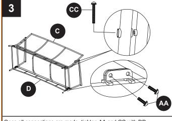
Once all connections are made, tighten AA and CC with DD.
