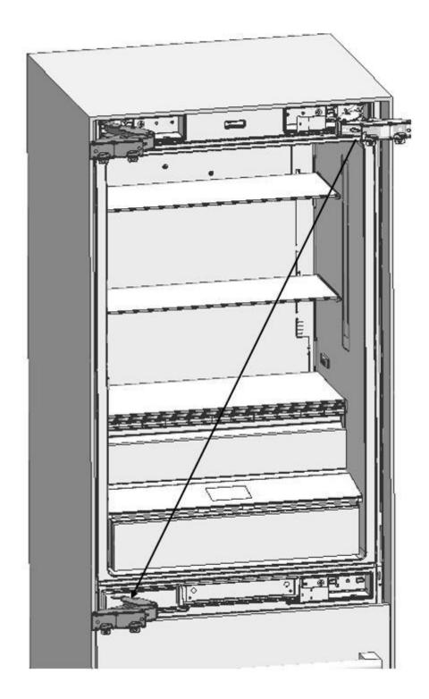
• Attach the Hinge Slot Caps removed from the left side to the Hinge Caps at the right side.
