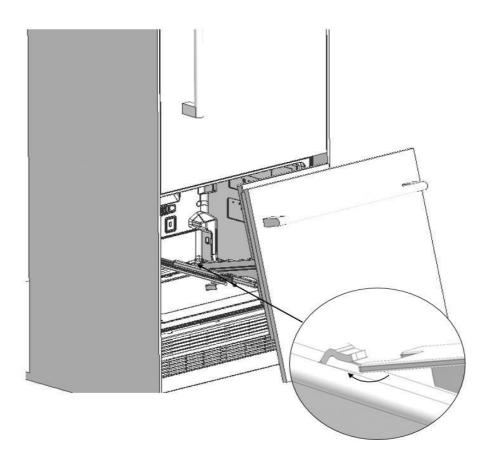
• Fix the Freezer Furniture door assembly onto the rails with 2 screws.
