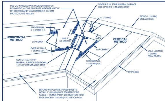
Mineral Guard® Roll Roofing can be installed following either the Horizontal Method (parallel to the eaves) or the Vertical Method (parallel to the rakes). (See Figure 1)
