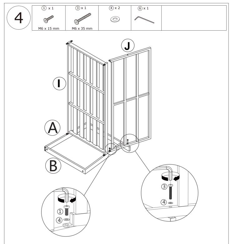
Fix part J with part A with one M6x35mm Screws (3)
