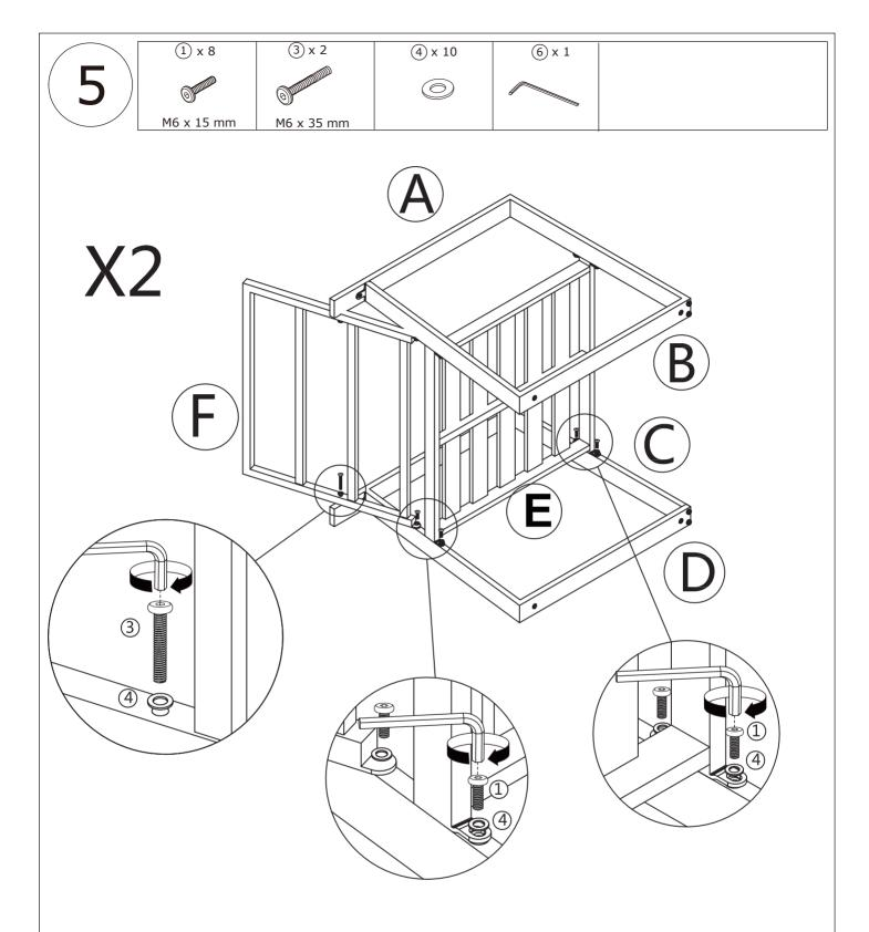
Fix part F with part C with one M6x35mm Screws (3) and (4) Flat Washers.Use (6) Allen key. **DO NOT YET TIGHTEN.** Fix part E and part F with part C and part D with four M6x15mm Screws (1) and (4) Flat Washers.Use (6) Allen key.
