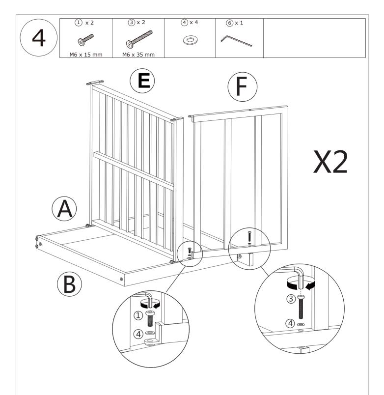
Fix part F with part A with one M6x35mm Screws (3)
