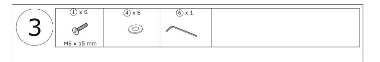
Fix part E with part A and part B with three M6x15mm Screws (1) and (4) Flat Washers.Use (6) Allen key. **DO NOT YET TIGHTEN.**
