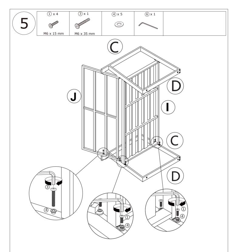
Fix part J with part C with one M6x35mm Screws (3)
