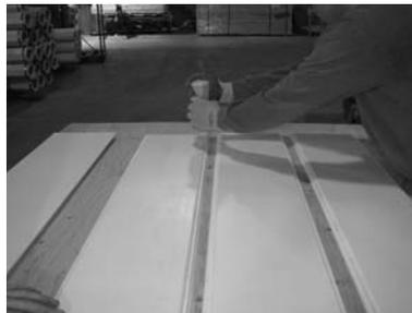
5) Lay 3 panels flat and apply adhesive to center joints.
