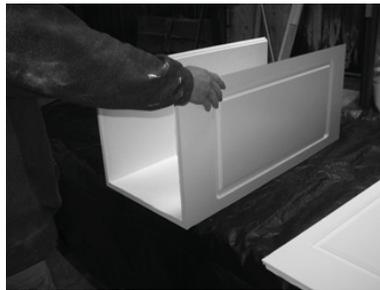
4) Assemble two panels to glued edges of panel from step 3.
