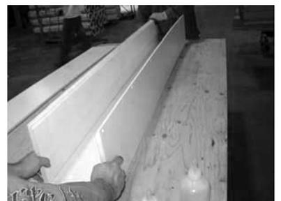
6) Assemble three panels, using E-Z Lock joints.
