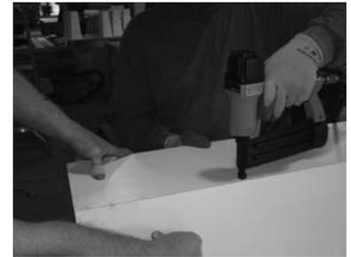
5) Pin-nail the three panels together into one unit. **See column instructions!**
