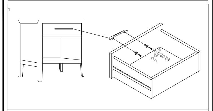
**Note:** Open the bedside cabinet and pull out the box, align the inner teeth of the cabinet pull rod with the holes on the bedside cabinet pull box, and use self tapping screws to pass through the holes from the inner surface and lock them in the inner teeth of the cabinet pull rod.
