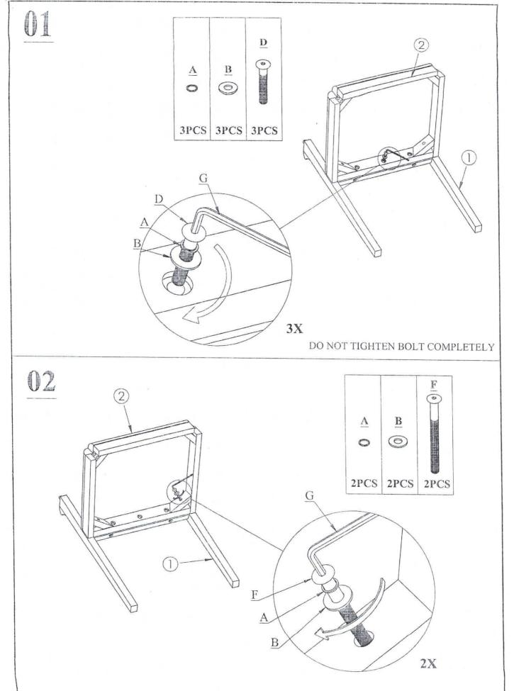
DO NOT TIGHTEN BOLT COMPLETELY
