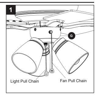
2. Using a ceiling fan will allow you to raise your thermostat setting in summer and lower your thermostat setting in winter without feeling a difference in your comfort. **Note:** Wait for the fan to stop before moving the reverse switch located on the light kit (G).
