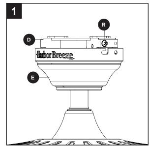
2. Secure the canopy (E) with the mounting bracket screws (R) previously removed (Step 4, page 8). Tighten all mounting bracket screws (R) securely.
