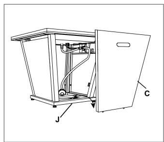
**6.** Attach hose of regulator tightly to the bracket.
