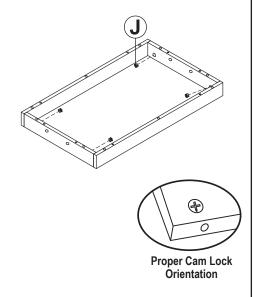
Align Cam Lock (J) with each cam screw; make sure the "C" shaped side of the cam lock fits over the head of the cam screw. Use a screwdriver to turn the cam lock until it locks onto the screw head.
