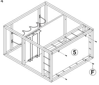
Slightly angle Bottom Shelf (5) between the middle shelf and bottom rails and place it on top of the metal tabs inside the bottom rails.
