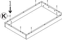
Insert 8x Dowels (K) into the Top Shelf End Panels (9) and Top Shelf Side Panels (10). Align Top Shelf (11) with the dowels, then secure using 10x Connecting Screw (H). Do not over-tighten.
