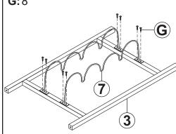
Secure 2x Bottle Rack (7) to Top Frame (3) using eight M4 x 14mm Round Head Screws (G).
