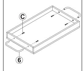
Securely fasten 2x Handles (6) to the end panels of the top shelf using four M6 x 25mm Bolts (C).
