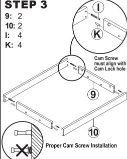
Insert 2x Dowel (K) into the bottom holes of each Top Shelf End Panel (9).
