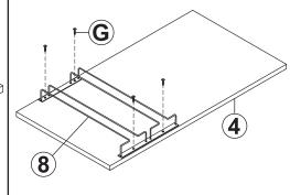
Secure Stemware Holder (8) to Middle Shelf (4) with four M4 x 14mm Round Head Screws (G).
