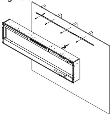
unit is an electrical appliance that is **NOT** watertight and must be installed as to prevent water from entering unit. This must be installed away from showers, tubs, etc. Never locate fireplace where it may fall into a bathtub or other water container.
