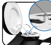
7 Lock the safety rope and connect the wires of the light.
