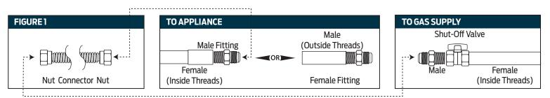
WARNING: Turn off gas supply before disconnecting old appliance. In absence of manual shut-off valve near appliance location, gas MUST be shut off on the main valve, near the meter.
