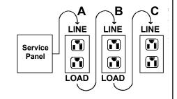
Placing the GFCI in position A will also provide protection to "load side" receptacles B and C. On the other hand, placing the GFCI in position C will not provide protection to receptacles A or B. Remember that receptacles A, B, and C can be in different rooms.
